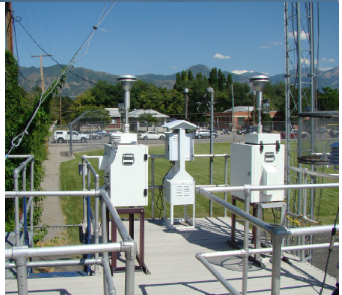
Air quality monitors measure PM 2.5 and other pollutants at several locations in the Salt Lake Valley.
